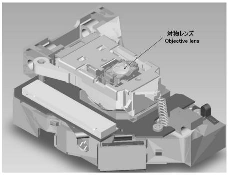
Fig.5-1 Optical pickup
