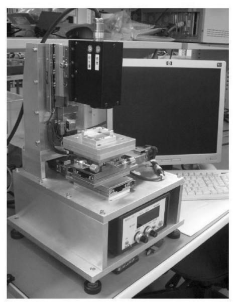
Fig.5-7 inspection system for OPU gluing
