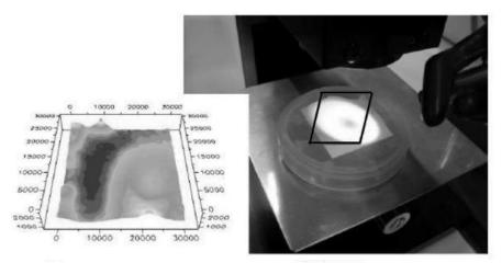
Fig5.13 Distribution of intensity of fluorescent light compared to the area of exposure
