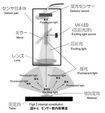
The way of measuring is very simple. You can measure just when you put it on the table of the sensor and focus the exciting light on. The diameter of the spot is  $\varphi 0.5$ ~2mm (refer to table 4.1).
