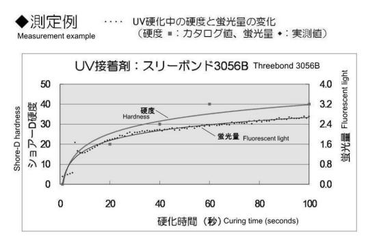
Fig4.4 Hardness of glue and the amount of fluorescent light
