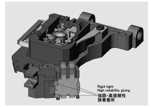
Fig.5-4 the gluing point of OPU (not for optical components)
