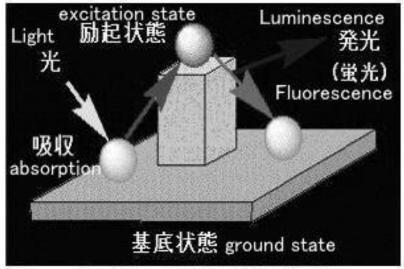
fig.2-1 Fluorescence, excitation and luminescence with excitation light
