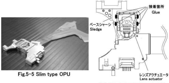
Fig.5-6 the glue points of Slim type OPU
