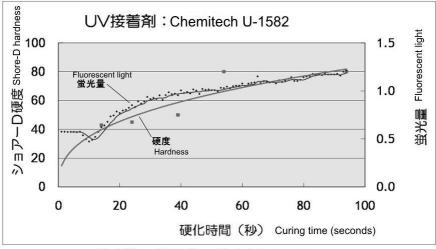
Fig4.5 the other example of UV curing glue
