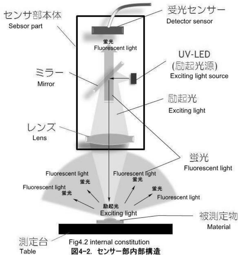
The way of measuring is very simple. You can measure just when you put it on the table of the sensor and focus the exciting light on. The diameter of the spot is  $\phi 0.5\sim 2\text{mm}$  (refer to table 4.1). The exciting light is invisible light, but it is easy to see the spot on a sheet of white paper or something as well. (Because white paper contains a lot of fluorescent material.) Please put protective glasses on.
