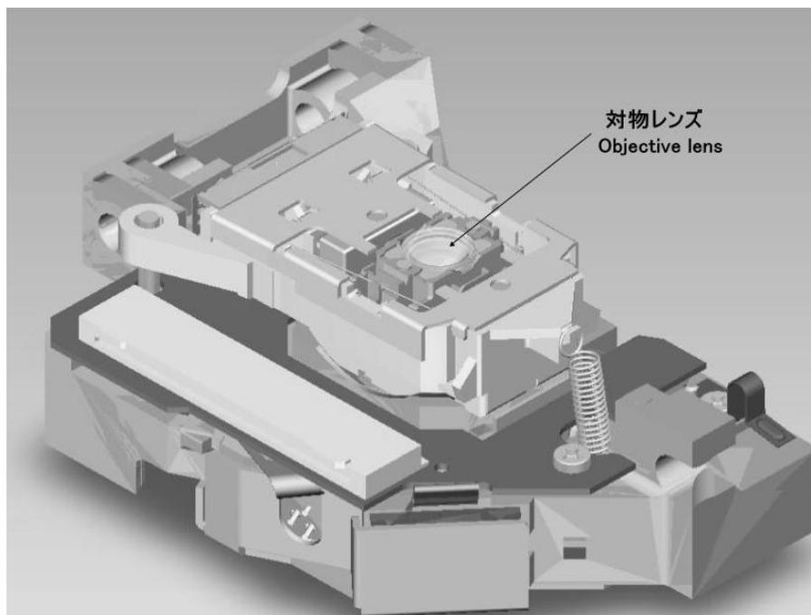
Fig.5-1 Optical pickup
