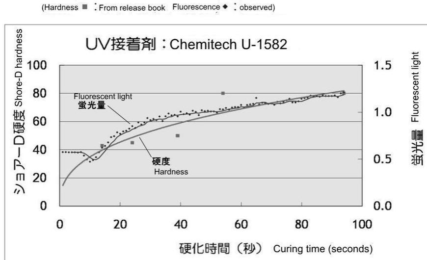
Fig4.5 the other example of UV curing glue
