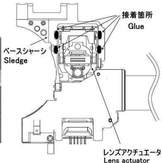
Fig.5-6 the glue points of Slim type OPU
