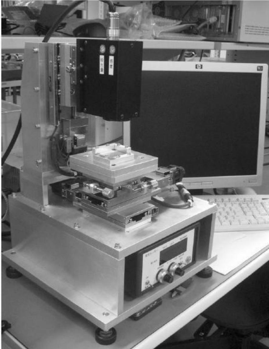
**Fig.5-7 inspection system for OPU gluing**
