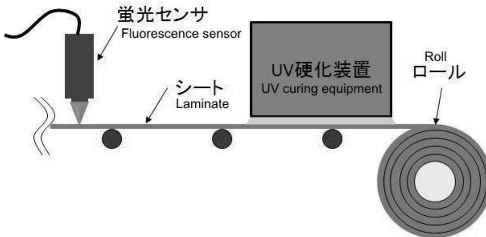
Fig5.10 Inspection of a roll of laminate in a factory
