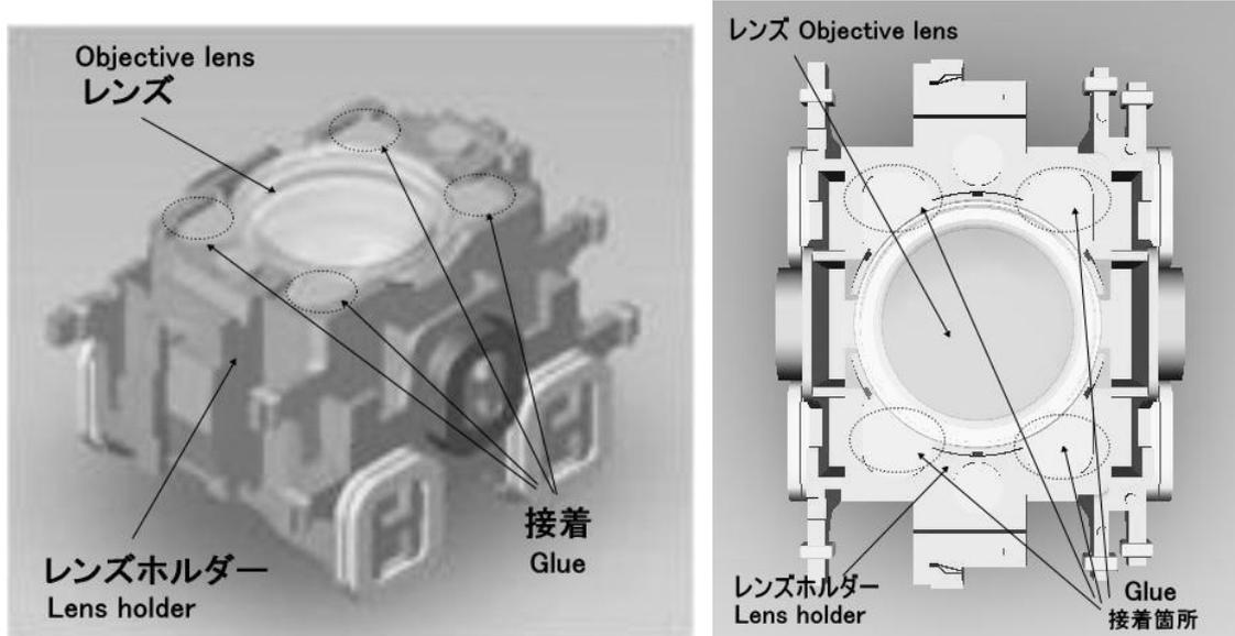
Fig.5-2 Objective lens and the lens holder of Optical pickup
