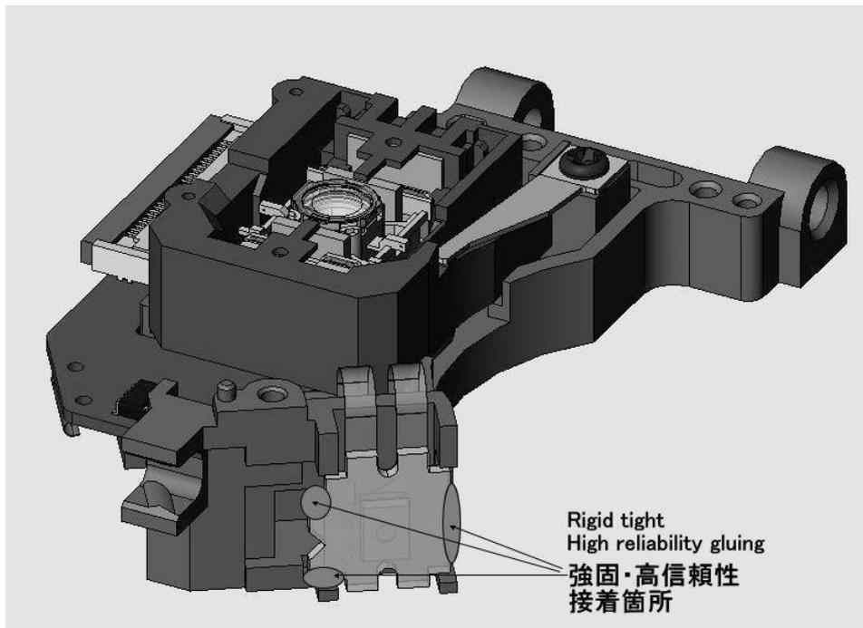
**Fig.5-4 the gluing point of OPU (not for optical components)**
