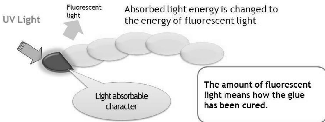
Fig3.5 The material changed to fluorescent material.
