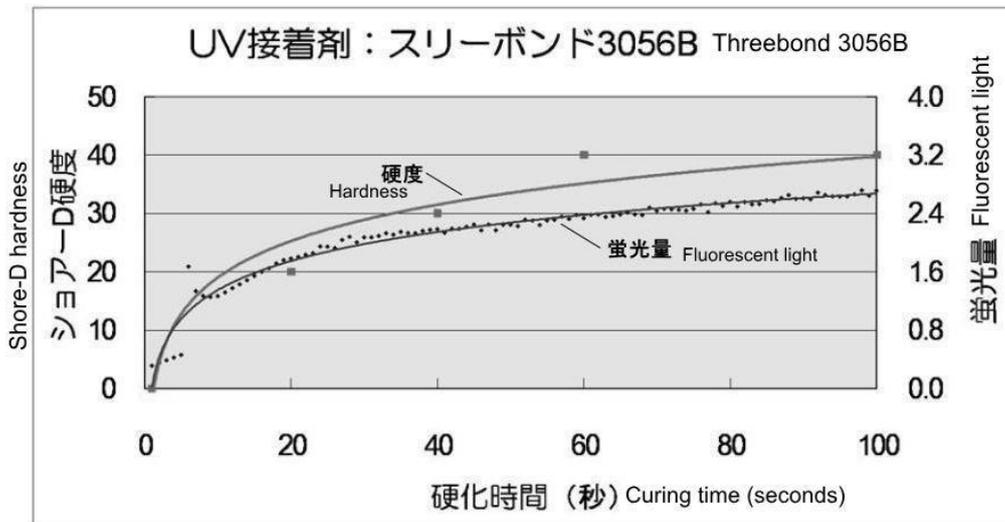
Fig4.4 Hardness of glue and the amount of fluorescent light
