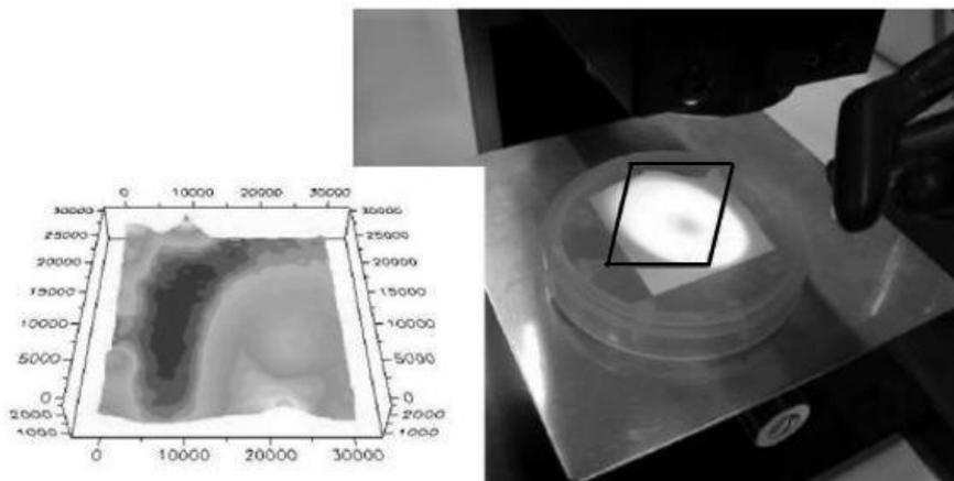
Fig5.13 Distribution of intensity of fluorescent light compared to the area of exposure
